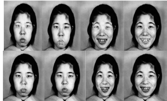
Fig. 7 Detected corner points on the facial feature and around the facial feature
